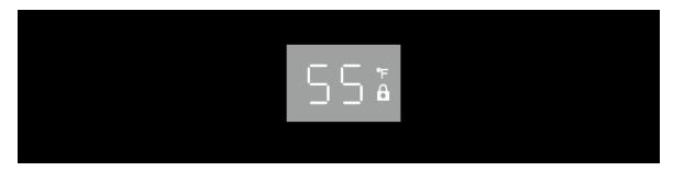
You also have the option of turning off the display temperature digits when the control panel goes to sleep, with the control panel locked, holding the LIGHT button for 3 seconds will cause the display temperature digits to darken (hide) in sleep mode. Holding the LIGHT icon again for 3 seconds will reverse this feature.
